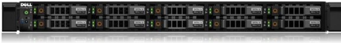
Figure 2. 10-drive bay chassis front view without bezel
