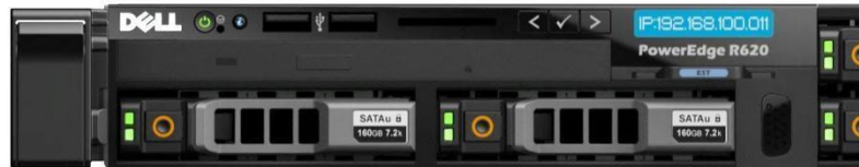
Figure 6. LCD control panel for 8-drive bay chassis
