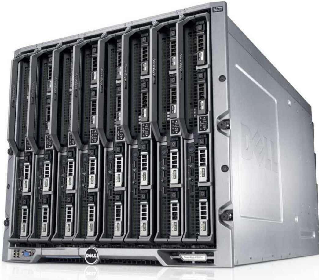
Figure 2. M1000e chassis enclosure with M820 blades
