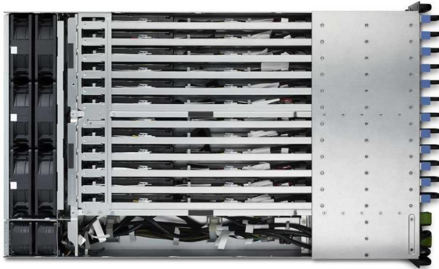
Figure 4. Internal view of the PowerEdge C5000 with PowerEdge C5220 servers
