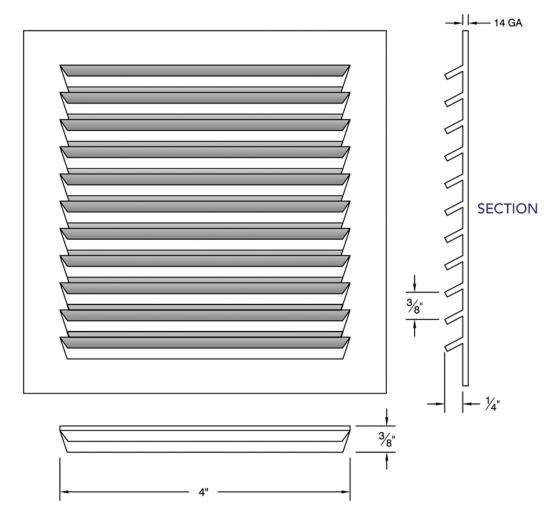
Consisting of multiple fixed blades, our punch louvers are ideal for air direction and flow in any interior or exterior commercial space.
