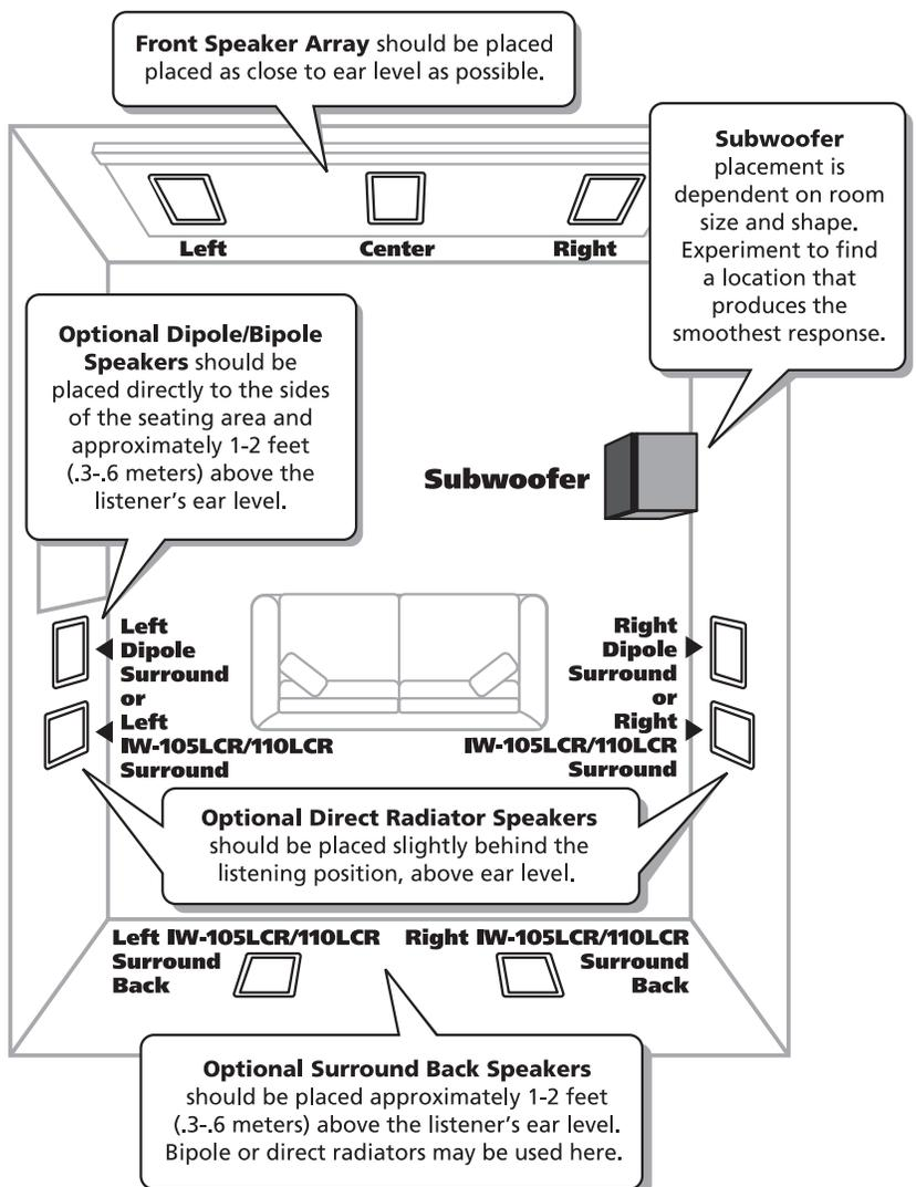
The spacing of the left-right speakers can be a little wider than with 2-channel stereo speakers, since in a theater system, the center channel speaker reproduces the on-screen effects and anchors the center image. Left-right spacing of about 8 to 10 feet usually works well.
