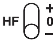
"+" is for absorptive, acoustically "dead" rooms (or when the speaker is behind a movie screen). Use this position to increase the HF level and restore the proper sparkle and liveliness to the sound.
