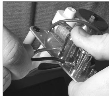
Strip about 1/2" (13 mm) of insulation from the connecting wires. Connect them to the appropriate push terminal, being careful to observe polarity (positive to the red terminal, negative to the black terminal).
