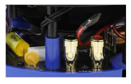
Atlantic's AZURE 20 series speakers feature computer optimized 12 dB/octave precision crossovers. The crossover is made using audiophile grade components including polypropylene capacitors, air core inductors and a built-in resettable polyswitch for speaker protection.
