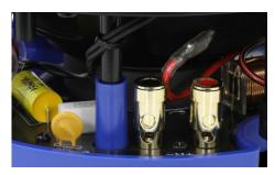
Atlantic's AZURE 10 series speakers feature computer optimized 12 dB/octave precision crossovers. The crossover is made using audiophile grade components including polypropylene capacitors, air core inductors and a built-in resettable polyswitch for speaker protection.
