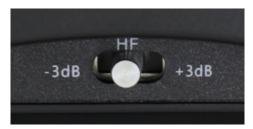
For further installation refinement, the AZ610/810 also include a front mounted +/- 3 dB tweeter level control using precision resistors for optimizing the speaker to its surroundings and adjusting for boundary reflections or absorbent materials.
