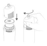
d. Install the suction nozzle on the transparent cover.
