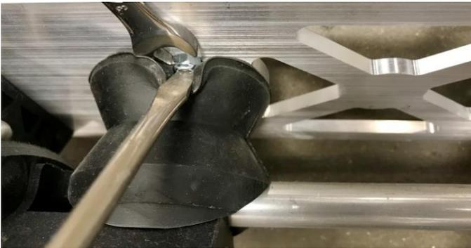
Next, remove the old Mechanism Plate from the Mechanism Tower. All hardware can be discarded. Inspect the Rubber. If it is worn and/or cracked, we recommend replacing it.
