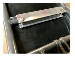
A bent plate is shown to the right. If necessary, you can straighten the plate or rivnuts with a set of vice grips. If you are still having difficulty, the holes in the Repair Channel can be drilled out to the next size up.
