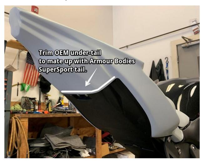
Simply use a Dremel tool and cut away the OEM under-tail piece where outlined. Test fitment is recommended as you cut to avoid removing too much of the undertail.
