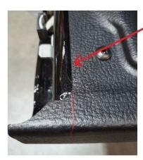
Close the tailgate and check your marking is straight and all the way around the edging of the Tailmate.
