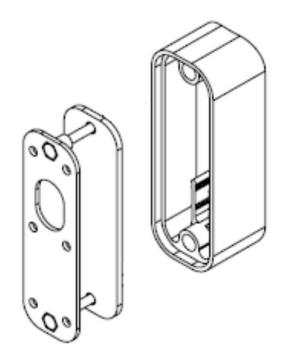
VIEW OF WALL FIXING PLATE COMPONENTS
