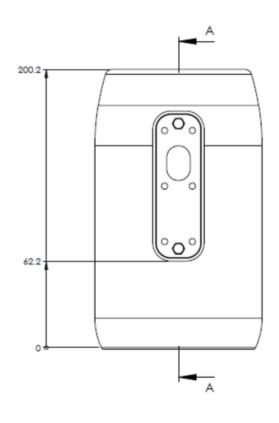
VIEW OF WALL FIXING PLATE FROM THE BACK
