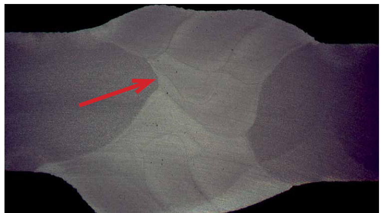
Figure 6-4: Cross section of weld showing lack of side wall fusion
