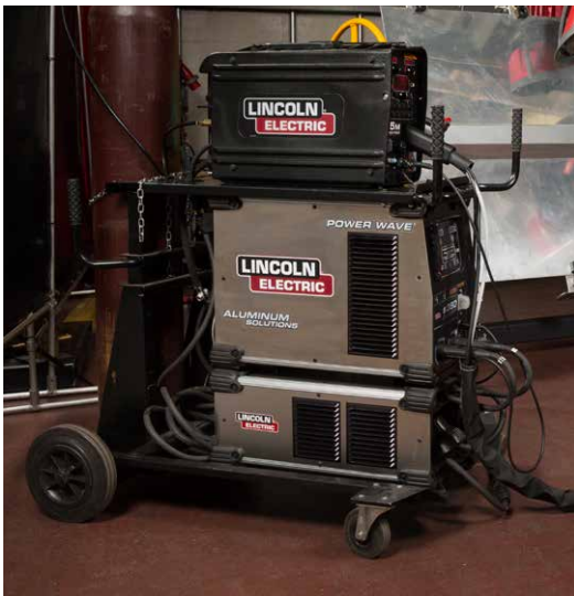
Figure 5-4a: Power Source with Advanced Module
