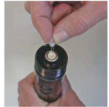
8. Insert pins of new "Bi-Pin" lamp into the two holes of the adapter. Do not bend or twist the lamp pins.
