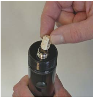
5. Insert the "Bi-Pin" lamp adapter (silver colored contact end in first).
