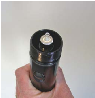
9. Make sure lamp is fully seated.
