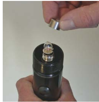
3. Remove the old retaining collar. You will be replacing this with the new collar.
