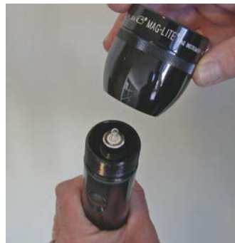
10. Place a small amount of petroleum jelly on threads and rubber O-rings and re-install head assembly
