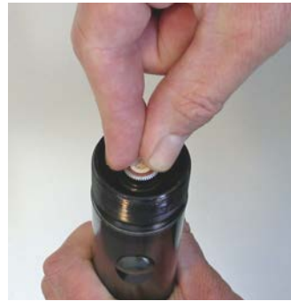
7. applying a slight amount of downward pressure to catch the threads. Hand tighten retaining collar.
