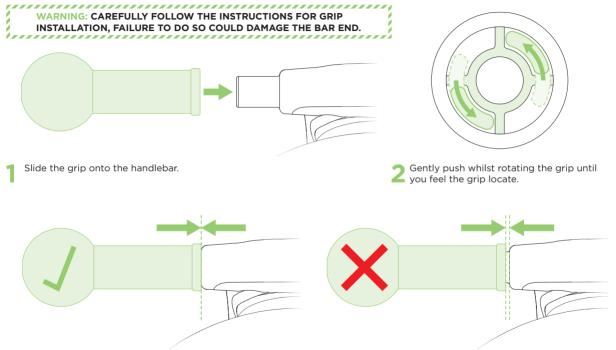
There should be no gap between the grip and the frame, and you shouldn't be able to rotate the grip. If there is a gap, then rotate the grip whilst pushing gently until the gap is closed, and the grip can't turn.
