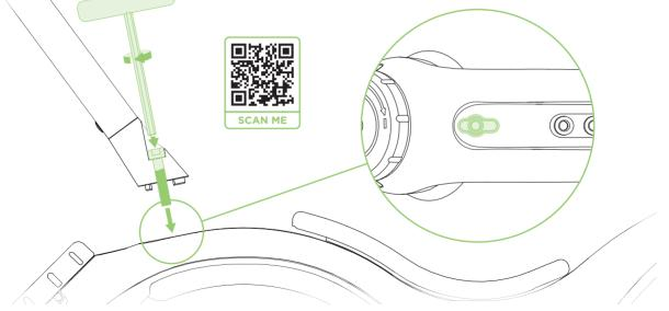
To attach, locate the tiller's end into the tiller mount on the frame. Using the 4mm allen key, secure the tiller to the frame with bolt provided, tightened to 2.5-3nm.
