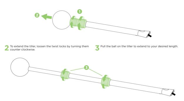
Tighten the twist locks by rotating them in a clockwise direction. Reverse these steps to shorten the tiller.
