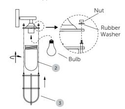
6. After installation, seal around the top and side perimeter between the fixture and the wall surface with weather resistant caulking. The bottom should be left un-caulked to prevent moisture build-up. Apply a small amount of weather resistant caulking around the side perimeter between the cap nut and mounting plate.
