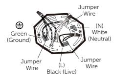
3. Connect (push) electrical stripping wires from the fixture (1) into the correct inserts. Black (live), White (neutral), Green (ground)
