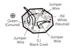
Connect (push) electrical stripping wires from the fixture (1) into the correct inserts. Black (live), White (neutral), Green (ground)
