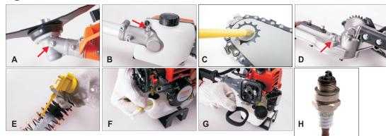
ABCDE: Apply 2-3 pumps of grease every 15 hours of operation.
