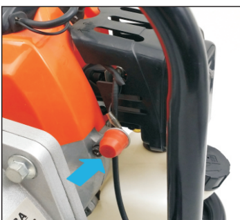
7. Pin the red button until engine totally stopped
