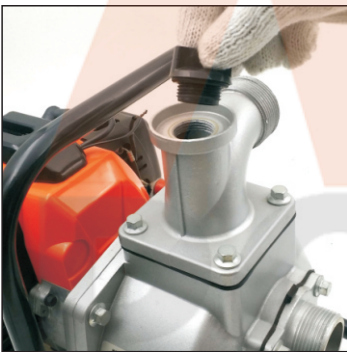
1. Unscrew cap and pour water into pump. The water level must be over mechanical seal, had better fill pump
