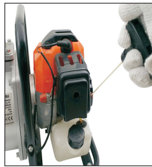
5. Pull starter again engine will be started
