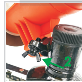
This knob for adjusting grinding depth
