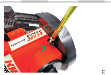
C: Lock the disc with pressing plate
