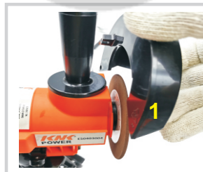
E: Mount disc cover 1 Thrust cover to groove 2 Screw up
