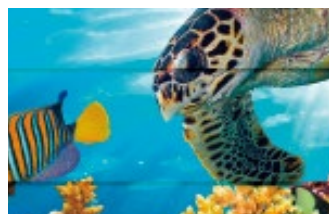
Overlap/Black streaks (Insufficient feeding amount)
