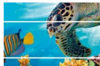
Gap/White streaks (Excessive feeding amount)
