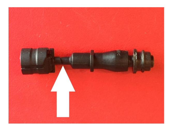
The part arrowed is the area inside which we are trying to clean, it is sealed and non removable, this is the part that will be damaged if a pin or needle is used.
