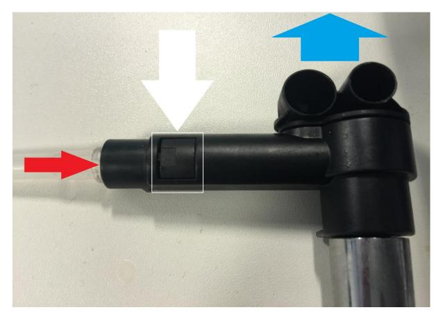
Remove the milk tube shown behind the red arrow.
