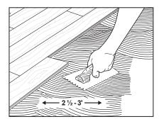
Secure your starter rows with a straight edge. Once the remainder of the floor has been installed, go back to the beginning and remove the straight edges and spread adhesive on the remainder of the open subfloor. Remember, planks closest to the wall may have to be scribed and cut to fit due to irregularities along the wall.
