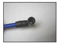
The steps for the HEI style terminals are similar to the conventional terminals except bending the HEI terminal is not required during insertion into the distributor boot.
