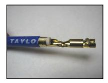
Next, carefully fold over the center core. Insert the wire into the terminal with the core next to the bottom of the terminal and form the terminal tabs around the wire to hold it in place for crimping.
