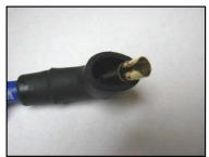
For the early style socket type terminal, put a slight bend in the terminal to aid in the boot installation. Insert the terminal/wire into the boot. Carefully bend the terminal up into a 90 degree configuration to fit the boot correctly. (You do not have to bend the terminal when using the late model HEI style boot/terminals).
