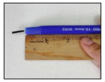
After you have measured and cut the wire(s) to the correct length, strip back 1/2" of silicone surrounding the center core. Next, shave approximately 3/4" in length and 3/8" in diameter at a tapered angle, being careful not to damage the core!
