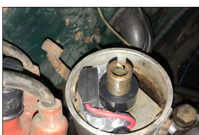
A Pertronix installed in one of my BMW 2002tiis. Photo by Rob Siegal
