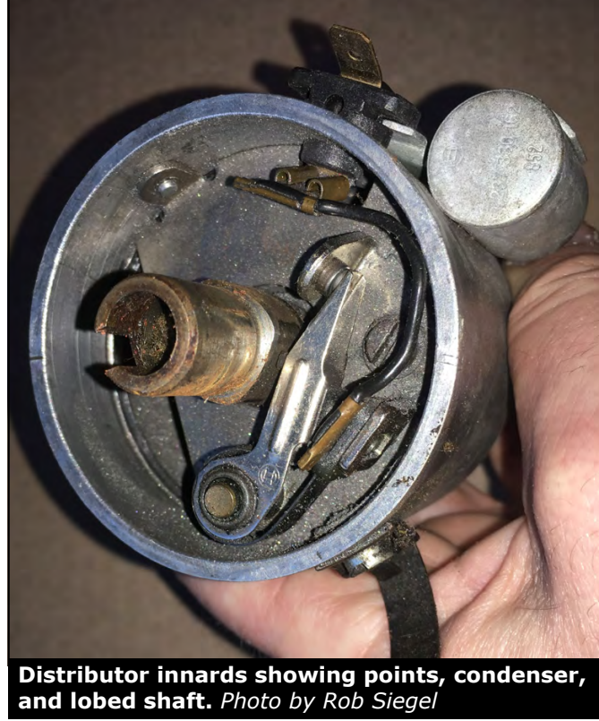
Distributor innards showing points, condenser, and lobed shaft. Photo by Rob Siegal
