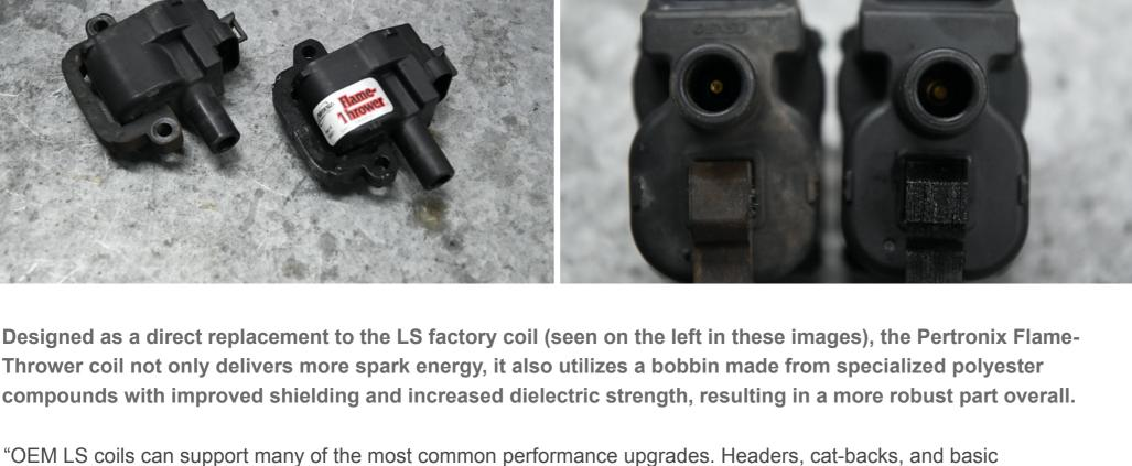
performance tunes are generally not enough to push OEM coils to their breaking point." That means that typical bolt-ons are fair game with the factory coils, provided they're functioning as designed. But the story changes a bit when more ambitious modifications are introduced into the mix.
