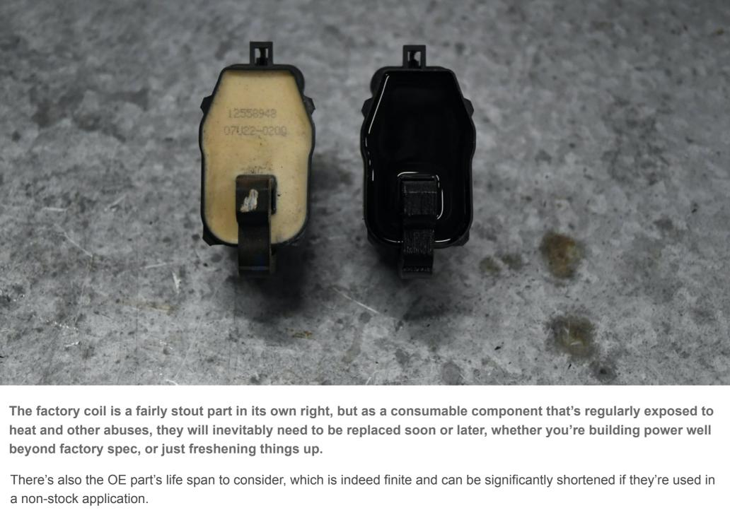
"Heat is a big killer of coils," Weaver notes. "Radiated heat from the engine can create external coil failures like broken connections, damaged wire insulation, failed electronic modules, and other issues. Excessive heat from the coils' operation can also damage the secondary windings. Coils operating beyond their design limits can cause internal breakdowns, too, and that can be triggered by conditions like extreme cylinder pressure and excessive spark plug gaps."
