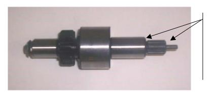
Remove material from these two surfaces as required to meet air gap of .075" - .125"
