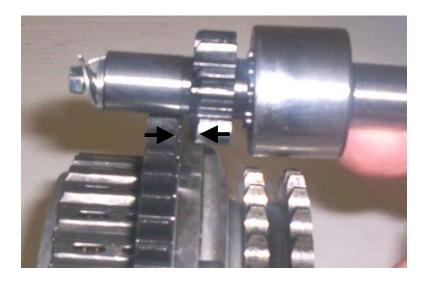
**Fig-1** (Adjust air Gap to .075" - .125")
