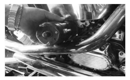
4. Clean the starter gearbox Housing where the starter mounts.
