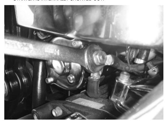
9. Reconnect the battery cables and test the starter. Never run a starter for more than 20 seconds at a time as this will overheat the starter and can cause it to burn out. If the bike does not start within 20 seconds, allow the starter to cool before trying again.
