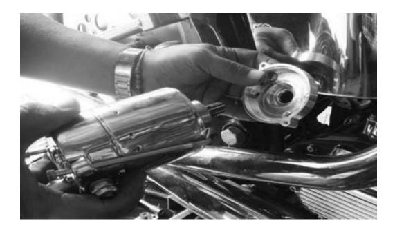
6. Install the Compu-Fire front housing to the starter gearbox on the primary. There are four sets of holes and two sets of screws. Orientate the holes that will allow the starter to be installed with the battery post in the same location as the original starter. Use the supplied screws that match the thread in the starter gearbox on your bike.
