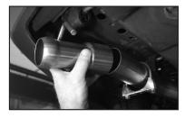
13. Install the passenger side tail pipe with tip hangers into the rubber isolators. Then slip into the muffler.
