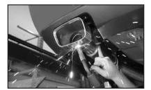
22. Check all clamps and connections for proper fit and alignment. Double check all clamps are tightened and that all hangers are secure in rubber grommets. It is recommended that after installation of the exhaust system you have all slip connections tack welded by a muffler shop. Using a soft cloth, remove all prints from exhaust.
