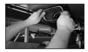
21. Tighten clamps, Tack weld slip connections, and ball clamp, to retain position of tip.
