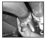
11. Slip the supplied clamps over the end of the X-pipe. Then install the new JBA mufflers on the X-pipe.
