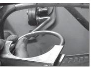
11. With rod pointing toward driver's side, install rear muffler clamp/hanger into lower hole of rubber grommet.
