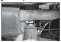
4. With muffler properly supported, using a reciprocating saw or hack saw, cut tail pipe off 5" behind rear of muffler.
