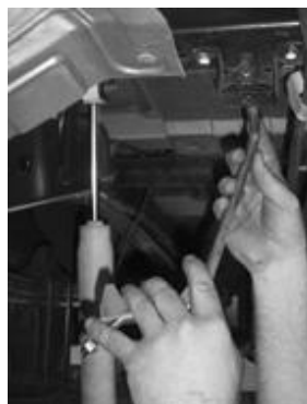
15. Install the JBA muffler (Muffler is oval, not round as shown) (D) on to the intermediate pipe (C)
