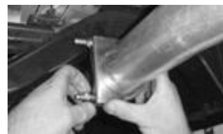
14. Install the 3" clamp with hanger (I) in to the rear muffler hanger grommet.
