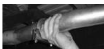
13. Install the JBA intermediate pipe (C) on to the resonator assembly and fit 3" clamp (I) over slip connection.
