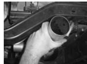
9. Fit the center exhaust hanger rubber grommet on to the hanger attached to the Y-pipe assembly (B). Then reattach it to the frame.
