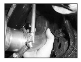
14. Slide the supplied 2-1/2" exhaust clamp on to the turn up pipe.
