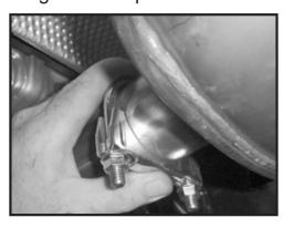
12. Slip the rear offset end of the JBA muffler (into the muffler clamp with hangers. The offset end of the muffler should be toward the center of the vehicle.
