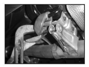
6. Unbolt the intermediate pipe from the catalytic converter assembly. \*\*\*Save the factory hardware for use later in the installation.
