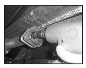
7. Using channel lock pliers remove the rear muffler hangers from the (2) rubber isolators and remove the intermediate pipe / muffler assembly from the vehicle.
