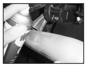
4. Unbolt the factory tail pipe above the rear axle.
