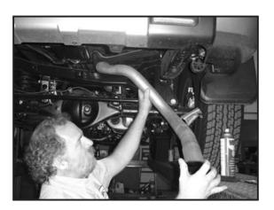
5. Using channel lock pliers pry the intermediate pipe hangers from the factory rubber isolators.
