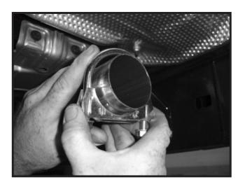
10. Install the muffler clamp with hangers into the rear (2) muffler hanger rubber isolators with the hangers shifting pipe to driver side.
