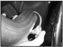
15. Install the tail pipe with tip onto the turn up pipe and insert hanger into the rear rubber isolator. Make sure to fully slide the two together for a tight seal and proper alignment.
