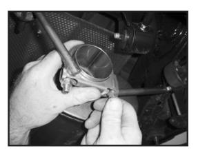
13. Slip the turn up pipe onto the JBA muffler. Position muffler clamp with hangers over connection and tighten.
