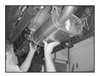
8. Insert the JBA intermediate pipe hangers into the (2) rubber isolators then bolt the intermediate pipe to the factory catalytic converter assembly using the factory hardware.
