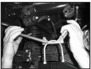
11. Insert the center inlet of the JBA muffler onto the intermediate pipe with the offset outlet closer to the center of the vehicle. Make sure to fully slide the two together and that the muffler is level and flat and tighten clamp over the connection.
