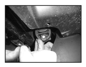
16. Make sure the new system is properly aligned and their is adequate clearance on the rear bumper then tighten the 2-1/2" exhaust clamp.
