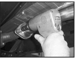
9. Slide one of the supplied 2-1/2" exhaust clamps over the end of the JBA intermediate pipe.
