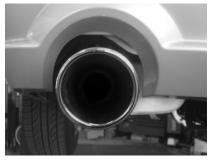
6. With the axle pipes in the muffler assemblies adjust mufflers to be flat, and the tips an equal distance from the bumper cover, Then tighten all clamps securely.
