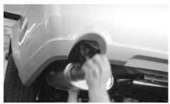
3. Using pliers or a pry bar, slide the rubber hanger from the hanger rod at inside, front of muffler (a little lube helps). Slide the muffler assembly forward and remove from slip hangers.
