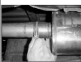
15. Install clamp (D) onto rear of muffler (#).
