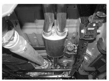
11. Align the chrome tip pipe so that it clears the body and looks astatically pleasing. Once you are satisfied with the position, tighten the clamp.
