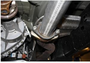
7. Slip the clamps over the inlet side of the tailpipes. Slip the pipes onto the over axle pipes.
