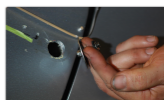
Use the Hardware provided with the Large washers for the two large holes in the body. It should look like this
