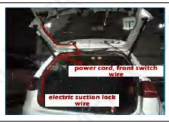
8. Route the power cable, CAN cable and front switch cable to the left side of the steering wheel and route the electric suction cable to the left side of trunk.
