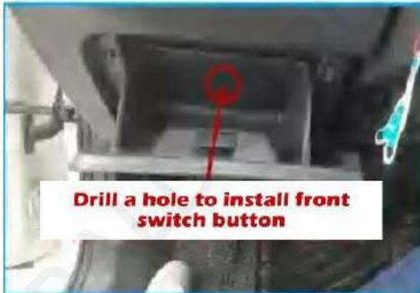
9. Punch a hole by 22mm drill to install our front switch.
