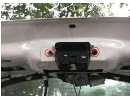
15. Install our electric suction lock and fix it with screws
