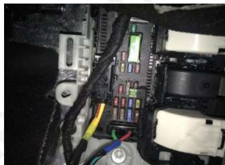
11. Take electricity from the co-pilot of the original car
