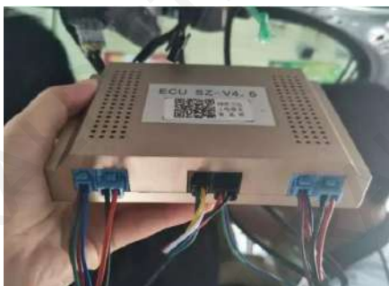
17. Hall wire, central control wire and power wire are plugged into our control box one by one according to the color
