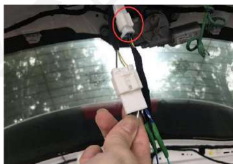
16. Plug the electric lock plug
