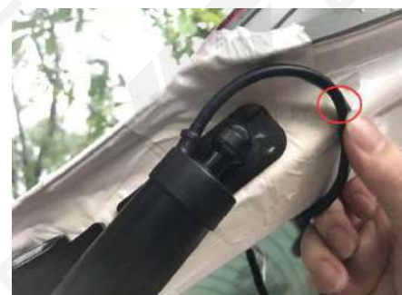
9. Punch at the top left (For poles wire ruote)
