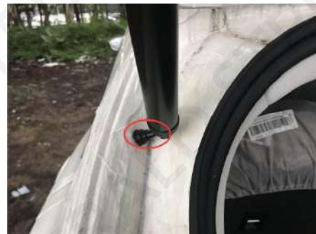
7. Install the left lower pole with the original car ball head
