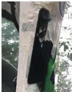
3. Install the upper left bracket of our company and fix it with flat screws
