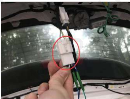
13. Connect the three-way wire
