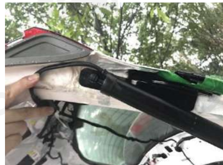
2. Remove the upper right ball head of the original car
