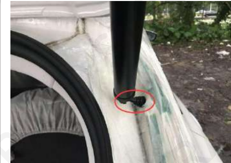
8. Install the right lower pole with the original car ball head
