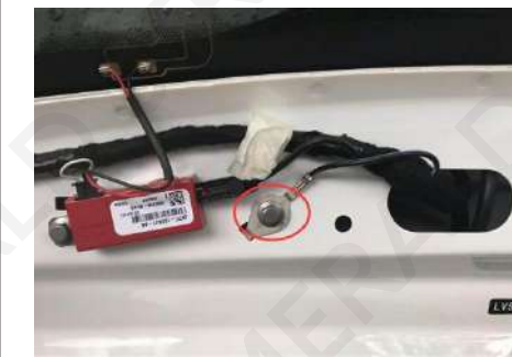
12. Ground at the rear of the car
