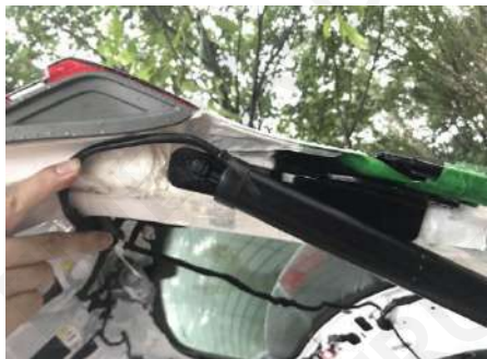
1. Remove the upper left ball head of the original car
