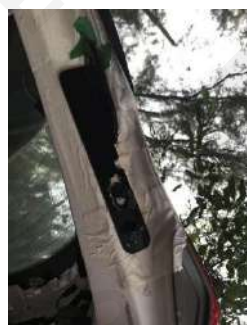
4. Install our upper right bracket and fix it with flat screws
