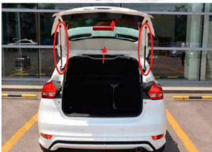
Remove the original car struts and trim
