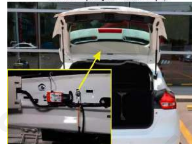
Find the grounding metal at the back door of the car and connect the power ground wire of our company.
