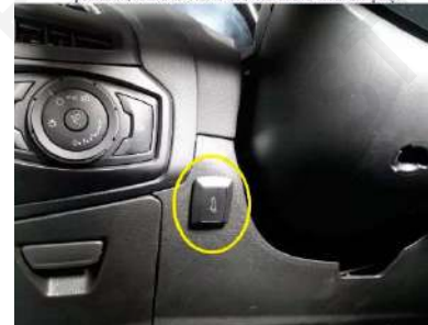
The main driver removes the trim and punches it, and installs the front switch button of our company.
