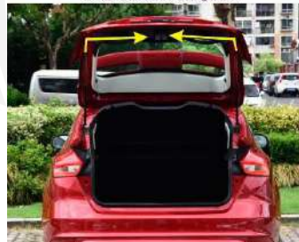
Punch holes above the ball head of the strut, and the strut line passes through the reserved hole inside to the tailgate cover.
