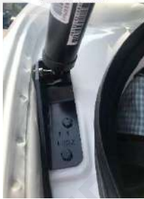
Remove the left lower bracket of the original car, install our left lower bracket and fix it with our screws.
