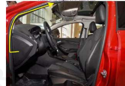
Power cable and front switch cable are routed to the tailgate cover control box
