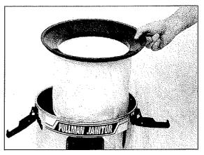
6. The filter can be taken out and cléaned, **Do not replace if using for wet pick-up**, only replace for dry use.
