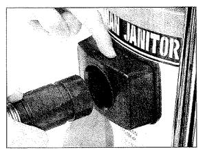
4. Fit the end of the hose into the input of the cleaner. Remove by pressing button as shown and pull hose out.
