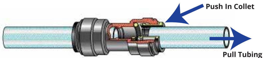
How to Use Quick Connect Fittings
