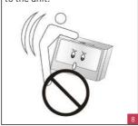
Do not move the product while it is switched on, as this may cause a fire and/or an electric shock.
