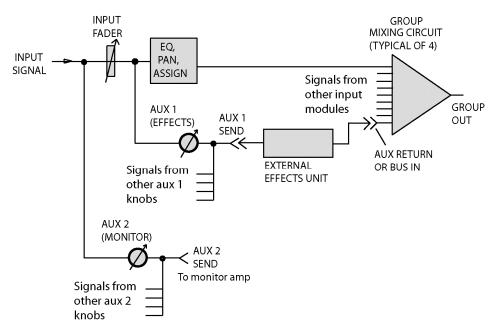
So, if you turn up the AUX2 knobs for the guitar, bass and drums, the AUX2 bus will contain a mix of those three instruments. On the back of the mixer is a connector labeled AUX2 OUT. If you plugged in an amplifier and speaker there, you'd hear the mix of guitar, bass and drums.
