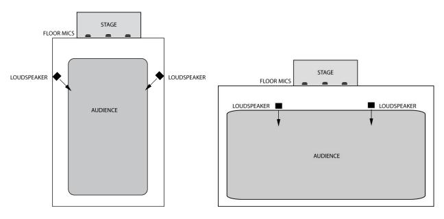
**Loudspeakers near the stage tend to cause feedback.** Then why are many auditoriums designed with the loudspeakers installed there? Those sound systems were designed for close-miked performances, in which feedback is not a problem. However, distant miking with floor mics requires a different speaker placement to minimize feedback.
