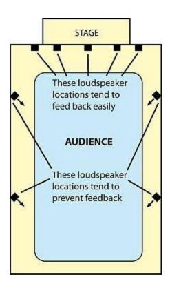
As a side benefit, the direct-to-reverb ratio of the loudspeakers' sound increases as you place the loudspeakers closer to the listeners. That improves intelligibility by reducing the perceived reverberation which smears syllables.
