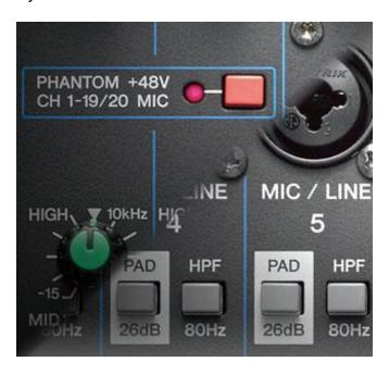
For example, "phantom power". Condenser mics need power to operate their internal electronics. That power can come from an internal battery, or an external voltage source such as a mixer, mic preamp, phantom power supply or audio interface.
