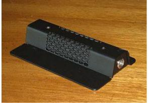
One effective way to pick up actors on stage is to use one or more stage-floor microphones, also called "area mics". Such a mic has a cardioid or supercardioid polar pattern, and is designed to be placed on the stage floor, about 1 foot from the edge, to act as a boundary microphone.
