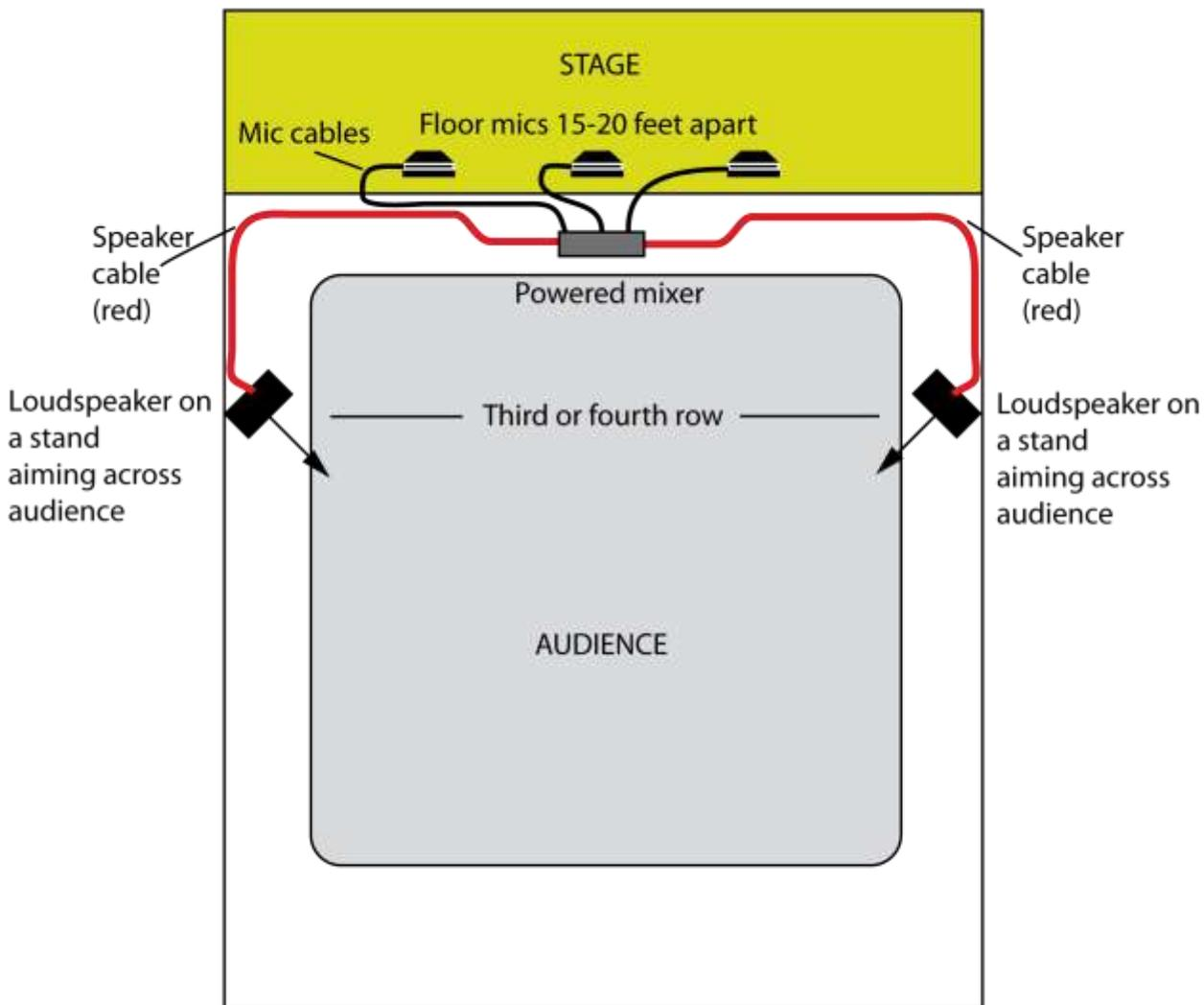
The mic cables plug into the powered mixer.
