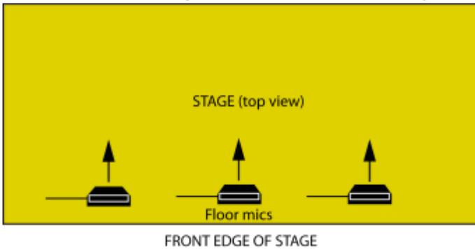
Connect each microphone to a long mic cable -- long enough to reach from the stage to your mixer. Your school or church might already have mic cables. You can connect several cables end-to-end to make a long cable run. Or you can use a **mic snake**, which is a metal box with several mic connectors and a long, thick cable going to the mixer.
