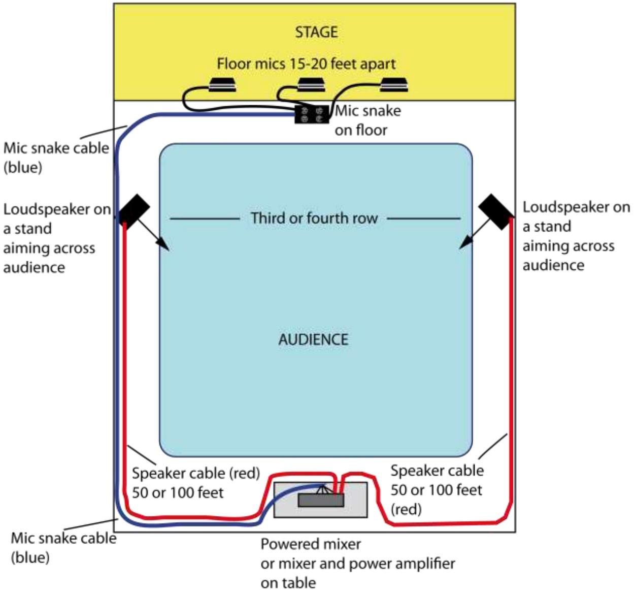
Connectors from mic snake plug into powered mixer.
