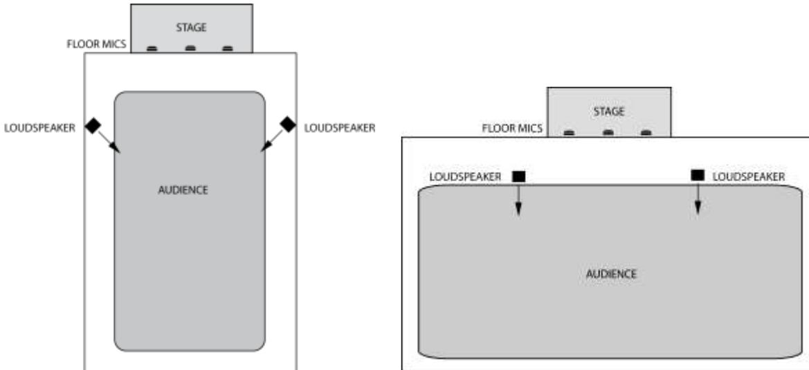
**Loudspeakers near the stage tend to cause feedback.** Then why are many auditoriums designed with the loudspeakers installed there? Those sound systems were designed for close-miked performances, in which feedback is not a problem. However, distant miking with floor mics or hanging mics requires a different speaker placement to minimize feedback.
